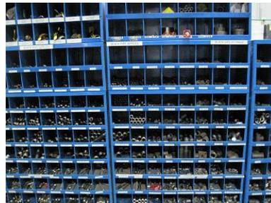
Storage bins directly under the LED fixture. Notice the vertical light in the "depth" of the light making for easy reading of part numbers.
