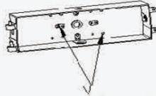
1. Open fixture by loosening two (2) screws located on the side, to install the power supply box onto the mounting surface. (Note: Don't drop screw)
